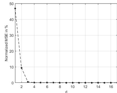
Figure 2: Leave-one-out MSE versus the number  $d$  of components considered in the 3D surrogate modelling procedure.
