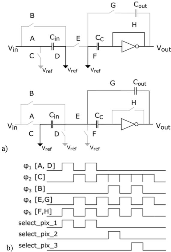
**Fig. 6** (a) Schematic of a switched-capacitor circuit able to perform positive and negative accumulations of a voltage value. Top : forward charging phase. Bottom : transfer phase. (b) Corresponding timing diagram of the control of the analog accumulator for a [2 -1 -1, 0 0 0, 0 0 0] mask.  $\phi_1$  controls switches A and D,  $\phi_2$  controls C,  $\phi_3$  controls B,  $\phi_4$  controls E and G, and  $\phi_5$  controls F and H
