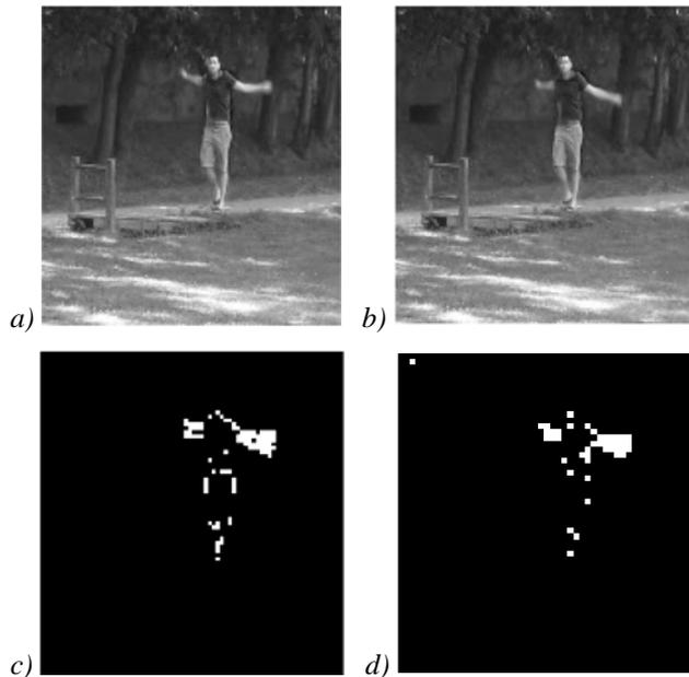
**Fig. 3** Temporal difference: (a) image from a video of a walking and waving man, (b) following image of the video, and thresholded differences of the two previous images with (c) a 1/(2x2) down-sampling or (d) a 1/(3x3) down-sampling. (a) and (b) have a resolution of 240x320 pixels, and so (c) is 120x160 and (d) is 80x107 pixels
