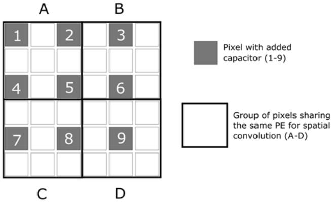
**Fig. 5** Schematic representation of the 6x6-pixel basic unit of the proposed matrix: 1 PE for 3x3 pixels, and 1 capacitor for 2x2 pixels. This should be replicated as much as necessary to build the whole matrix. The table presents the four PEs of a 6x6-pixel scheme and the pixels with added memory that they respectively manage during a temporal difference. Note that capacitor 5 of the pattern is to be connected to the “D” PE so that each PE manages 3 capacitors at the most
