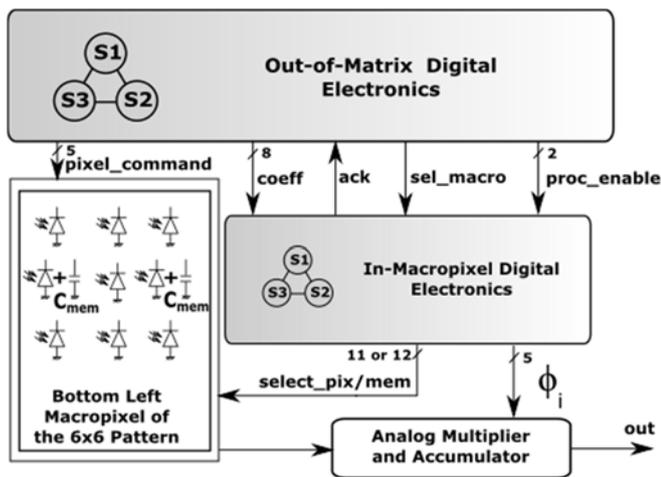
**Fig. 7** Schematic representation of the proposed sensor: out-of-matrix digital electronics control a macropixel PE, composed of digital control interfaced with the general out-of-matrix control, and an analog operative part: 1 multiplier and 1 accumulator per macropixel (3x3 pixels)
