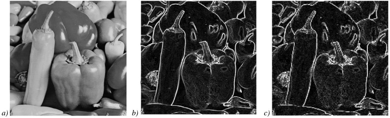
**Fig. 2** (a) Original image and (b,c) results of gradient computation using (b) classic convolution by a Sobel kernel (equivalent to 1 PE per pixel) and (c) down-sampled convolution with same kernel (equivalent to 1 PE per 9 pixels), performed on the classic image of peppers (512x512 pixels result in (c) 170x170 pixels)
