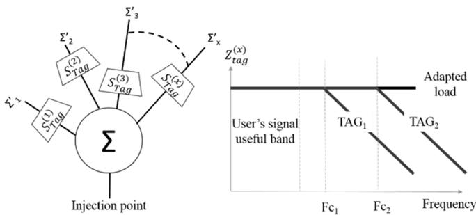
Fig. 2. Each extremity branch of a complex electrical network  $\Sigma$  is equipped with an electrical ‘‘tag’’ designed with a specific frequency pattern. As an example, the specific frequency signatures of the two TAGs were designed as low pass filters with two different cutoff frequencies outside the useful band.
