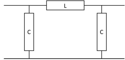
Fig. 3. Equivalent circuit of the electrical Tags inserted at extremities of the Y shaped network. The two tags are Pi Butterworth low pass filters with respective cutoff frequencies of 40 MHz and 65MHz.
