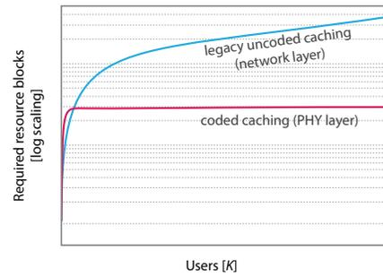
Figure 4: Required resource blocks for  $K$  mobile users with unicast demands, when the caches fit 30% of the catalog. Coded caching can serve an arbitrarily large population of users with a fixed number of resource blocks.
