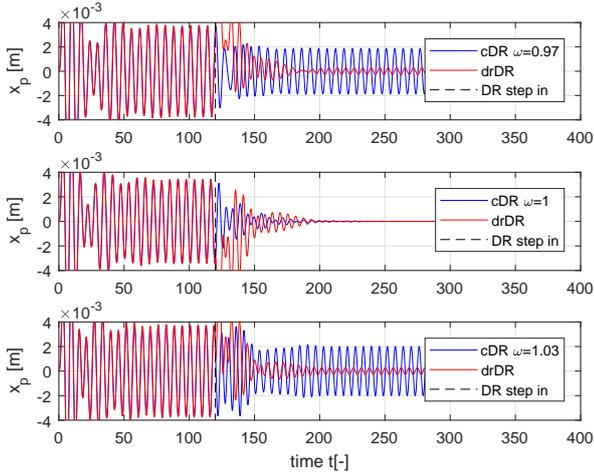
Fig. 4. Simulation results of delayed resonator performance at three excitation frequencies i)  $\omega = 0.97$ , ii) the nominal  $\omega = 1$  and iii)  $\omega = 1.03$ . Next to the results of the scheme with robust drDR (16)-(17) and the stabilizing controller (33) (red line), the results by the classical scheme with cDR with feedback (39) (blue line) are shown.
