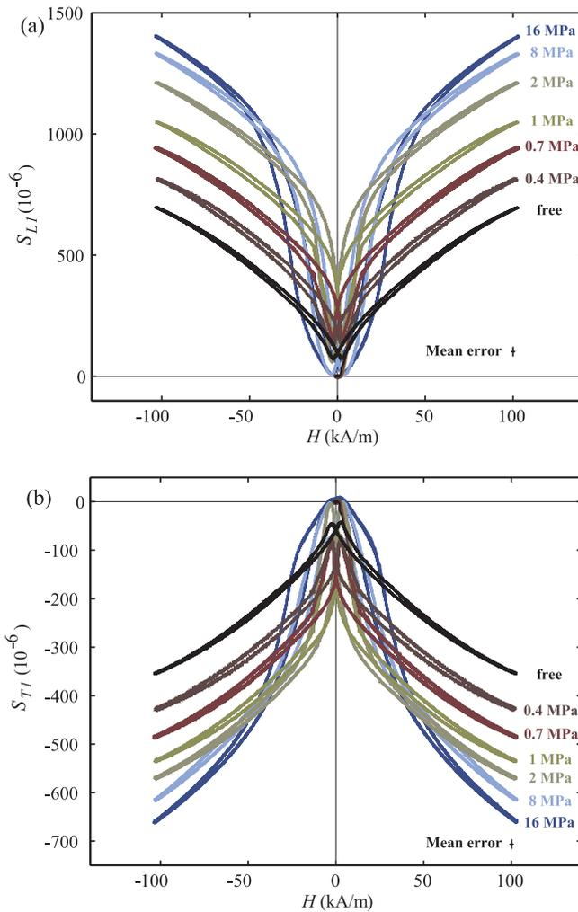
**Figure 4.** Longitudinal (a) and transverse (b) magnetostrictive behavior of a Terfenol-D specimen for various uniaxial applied compressive pre-stresses between 0 and 16 MPa under controlled stress conditions. The error bar on the measurement of strain and magnetic field is reported at the bottom right side of the graph.
