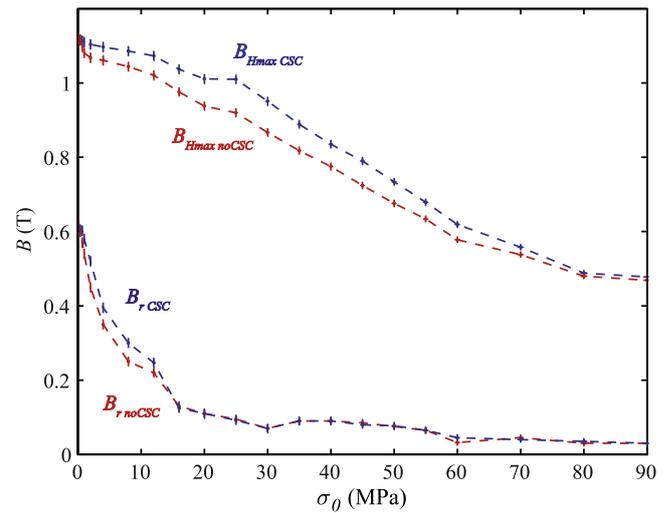
**Figure 9.** Evolution of remanent induction ( $B_r$ ) and induction at  $H_{\max} = 100 \text{ kA m}^{-1}$  magnetic field ( $B_{H_{\max}}$ ) versus compressive stress levels under controlled stress conditions (CSC) and uncontrolled stress conditions (noCSC). The error bars on the measurement of stress and magnetic induction are reported for each level of pre-stress.
