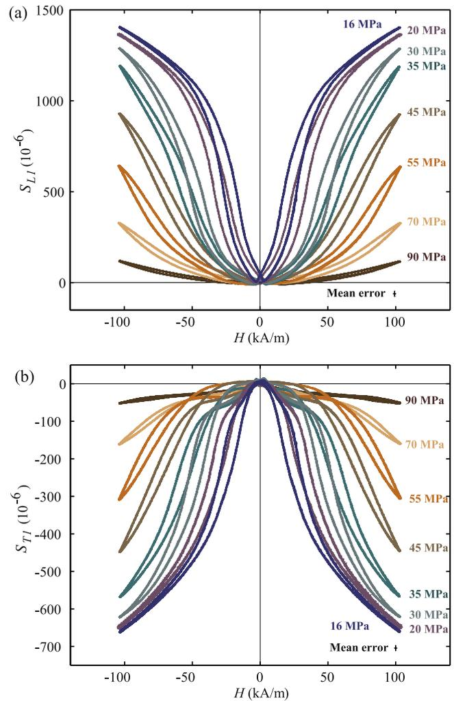
**Figure 5.** Longitudinal (a) and transverse (b) magnetostrictive behavior of a Terfenol-D specimen for various uniaxial applied compressive pre-stresses between 16 and 90 MPa under controlled stress conditions. The error bar on the measurement of strain and magnetic field is reported at the bottom right side of the graph.
