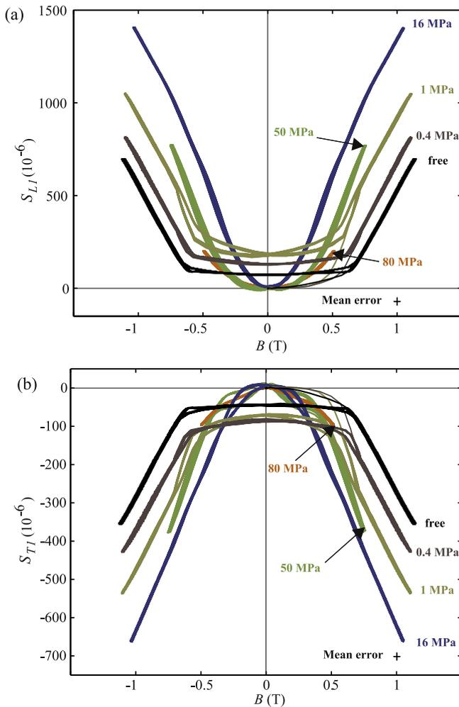
**Figure 6.** Longitudinal (a) and transverse (b) magnetostriction versus magnetic induction of a Terfenol-D specimen for various uniaxial applied compressive pre-stresses under controlled stress conditions. The error bar on the measurement of strain and magnetic induction is reported at the bottom right side of the graph.
