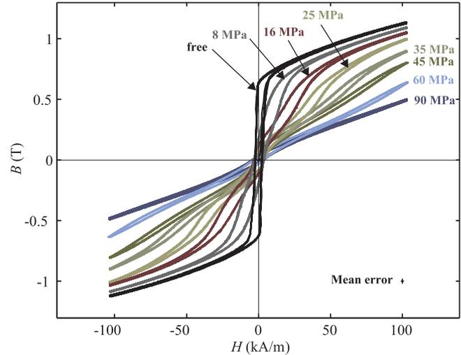
**Figure 3.** Magnetic behavior of a Terfenol-D specimen for various uniaxial applied compressive pre-stresses under controlled stress conditions. The error bar on the measurement of induction and magnetic field is reported at the bottom right side of the graph.
