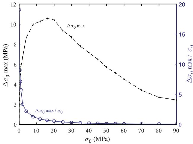
**Figure 8.** Maximum level of dynamic stress (dashed line) and associated ratio with the compressive stress level (plain line) during magnetic excitations under uncontrolled stress conditions. The error bars on the measurement of pre-stress and dynamic stress are reported for each level of pre-stress.
