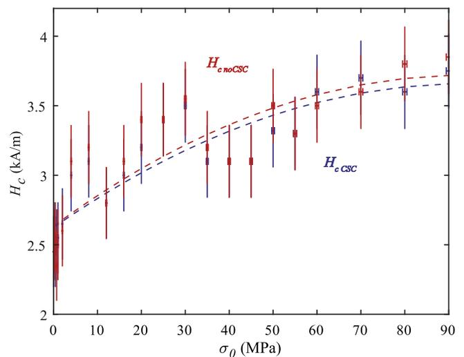
**Figure 10.** Evolution of  $H_c$  as a function of compressive stress under controlled stress conditions (CSC) and uncontrolled stress conditions (noCSC). The lines are just guides for the eye (polynomial regression, order 2). The error bars on the measurement of  $H_c$  and stress are reported for each level of compressive stress.
