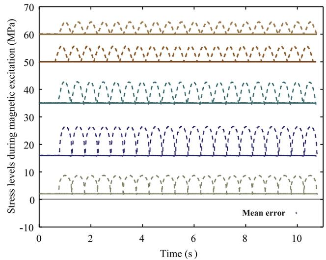
**Figure 7.** Stress levels experienced by the sample during magnetic excitation under 2, 16, 35, 50 and 60 MPa applied compressive stress: controlled stress conditions (plain line) and uncontrolled stress conditions (dashed line). The error bar on the measurement of stress is reported at the bottom right side of the graph.
