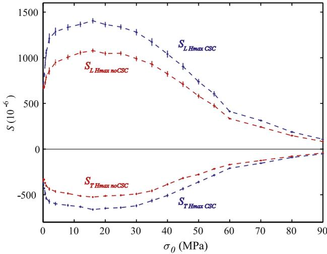
**Figure 11.** Evolutions of longitudinal and transverse magnetostriction strains at  $H_{\max} = 100 \text{ kA m}^{-1}$  ( $S_{LH_{\max}}$ ) and ( $S_{TH_{\max}}$ ) versus compressive stress levels under controlled stress conditions (CSC) and uncontrolled stress conditions (noCSC). The error bars on the measurement of stress and magnetostriction are reported for each level of pre-stress.
