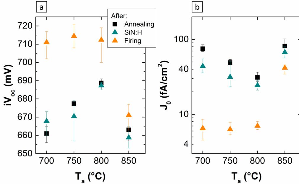
**Fig. 5.** Surface passivation properties ( $iV_{oc}$  (a) and  $J_0$  (b)) provided by the poly-Si(B)/SiO<sub>x</sub> structure as function of the annealing temperature  $T_a$ , evaluated on symmetrical samples (made from KOH-polished 156psq c-Si wafers) after annealing, SiN:H deposition and firing ( $d_{poly} = 20$  nm).
