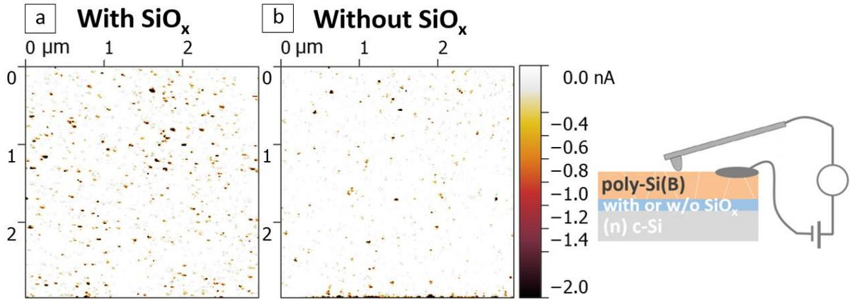
Fig. 9. Current maps obtained by C-AFM measurement in lateral configuration on 20 nm-thick poly-Si(B) layers ( $T_a = 700^\circ\text{C}$ ) with (a) and without (b)  $\text{SiO}_x$  layer at the poly-Si(B)/(n)c-Si interface. C-AFM measurements were performed 5h after HF-cleaning the samples' surface to ensure a similar surface state during both measurements.
