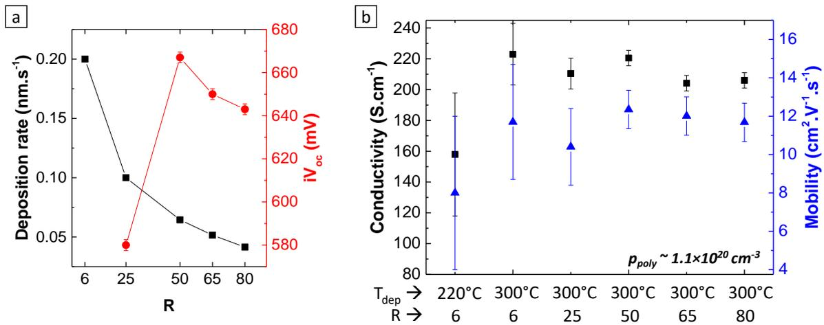
**Fig. 3.** Deposition rate of the a-Si:H(B) layer and *iV*<sub>oc</sub> (measured on symmetrical samples made from mirror-polished c-Si wafers) as a function of the gas flow ratio  $R = \text{H}_2/\text{SiH}_4$  (a). Conductivity and carrier
