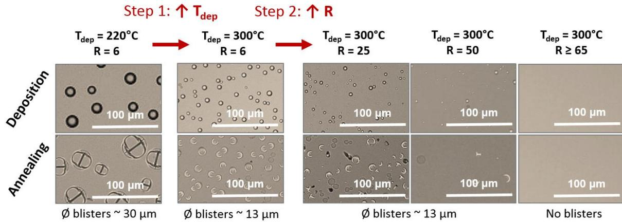
**Fig. 2.** Optical microscope images of 30 nm-thick poly-Si(B) layers after deposition and after annealing at 700°C (at a  $\times 20$  magnification). The deposition conditions were varied: **Step 1.** Increase of the deposition temperature  $T_{\text{dep}}$ , **Step 2.** Increase of the gas flow ratio  $R = \text{H}_2/\text{SiH}_4$ . For each set of conditions, the diameter of the blisters ( $\emptyset$  blisters) and their density were evaluated.
