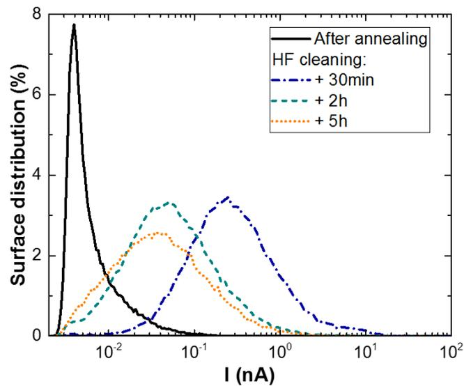
**Fig. 7.** Surface distribution of the detected currents extracted from C-AFM current maps measured at the poly-Si(B) surface in transversal configuration after annealing at 700°C and at different times after HF-cleaning the poly-Si(B) surface (from 30min to 5h).
