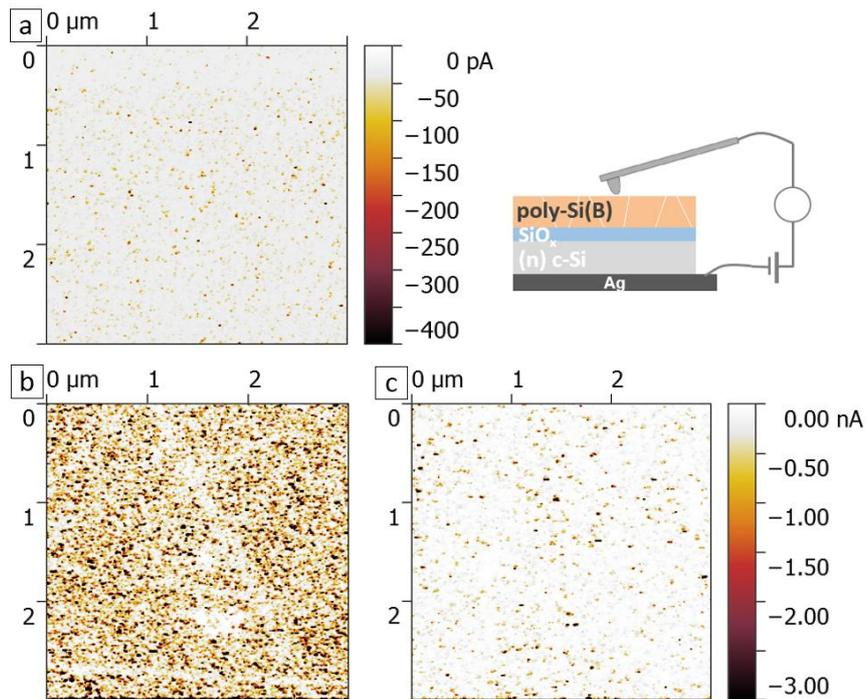
**Fig. 6.** Current maps obtained by C-AFM measurement in transversal configuration on a 20 nm-thick poly-Si(B) layer annealed at 700°C (a) and at different times after HF-cleaning the poly-Si(B) surface (30 min (b) and 5h (c)).
