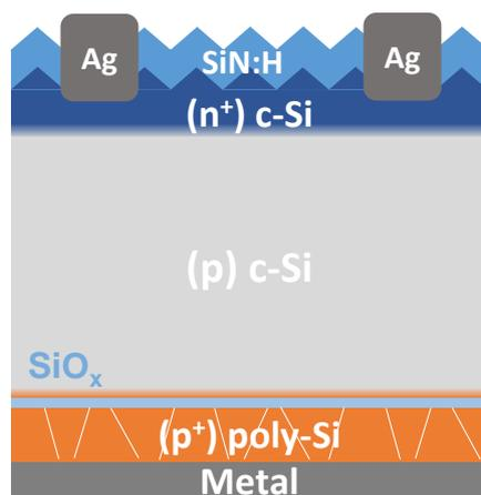
**Fig. 1.** Schematic of a p-type c-Si solar cell where the  $(p^+)$  poly-Si(B)/ $\text{SiO}_x$  structure discussed in this paper is integrated at the rear surface. The cell features a front  $(n^+)$  c-Si emitter that is coated with an anti-reflective hydrogen-rich silicon nitride layer (SiN:H). Local Ag metal contacts are formed on the front side. The rear contact consists of a full-area metal layer (e.g. Ag, Al).
