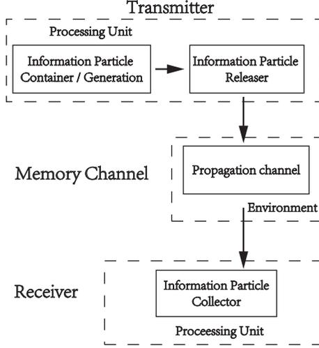
FIGURE 1: Block diagram of a typical MC system.
