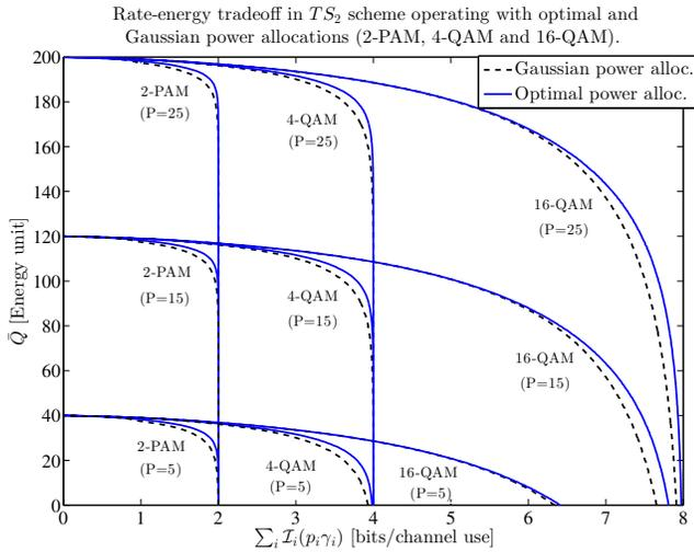
Fig. 10. Comparison of the RE trade-off in a SWIPT system employing  $TS_2$  with optimal and Gaussian power allocations for various signal sets and transmission powers. The system parameters are assumed to be  $N = 2$ ,  $|h_1|^2 = 4$  and  $|h_2|^2 = 1.2$ .
