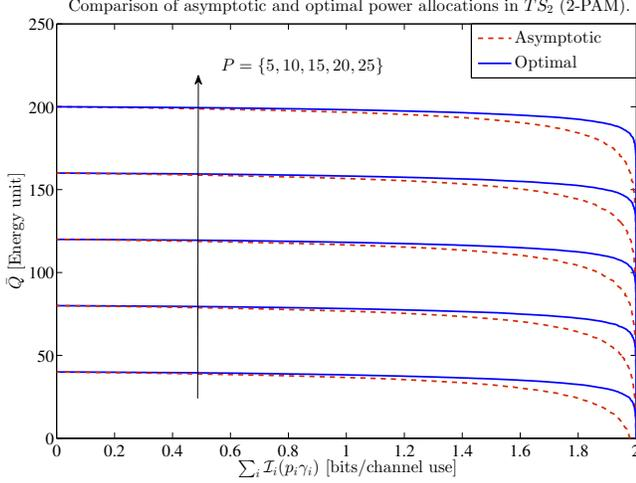
Fig. 7. Comparison of the achievable RE trade-off in a SWIPT system employing  $TS_2$  with optimal and asymptotic power allocations. The system parameters are assumed to be  $N = 2$ ,  $|h_1|^2 = 4$ ,  $|h_2|^2 = 1.2$  and 2-PAM signal set over both the channels.
