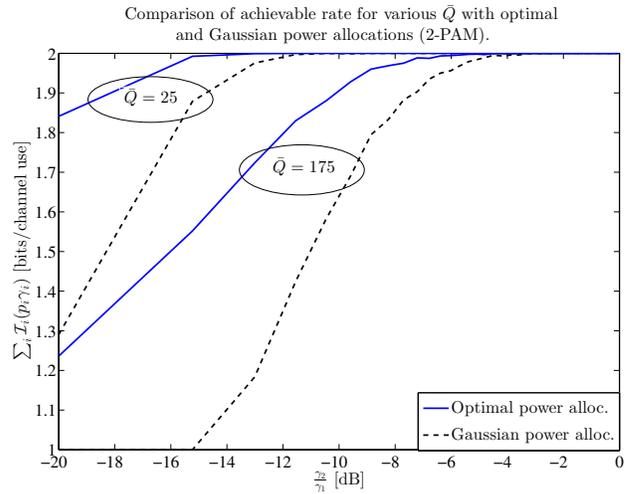
Fig. 11. Comparison of the achievable rate as a function of  $\left(\frac{\gamma_2}{\gamma_1}\right)$  in a SWIPT system employing  $TS_2$  with optimal and Gaussian power allocations. The system is assumed to operate with 2-PAM signal set over both the channels.
