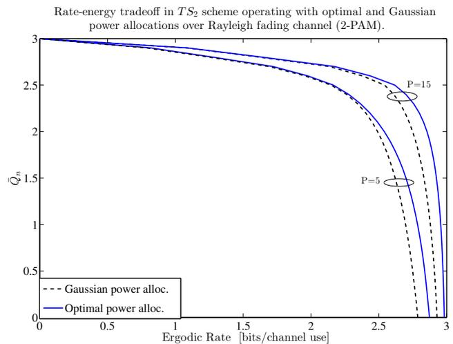
Fig. 14. Comparison of the achievable RE trade-off in a SWIPT system employing  $TS_2$  and operating over  $3 \times 3$  Rayleigh fading channel with the aid of beamforming. The system is assumed to operate with 2-PAM signal set over all the channels.
