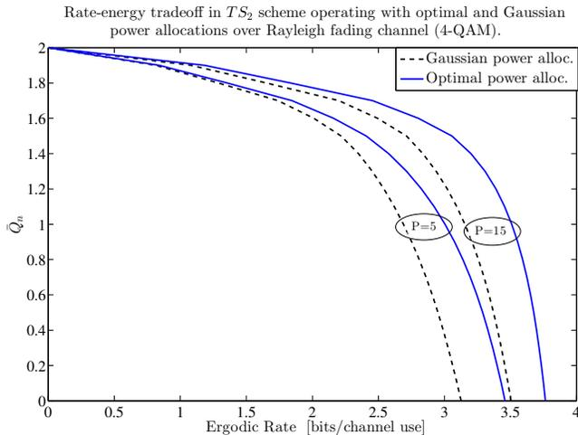
Fig. 13. Comparison of the achievable RE trade-off in a SWIPT system employing  $TS_2$  and operating over  $2 \times 2$  Rayleigh fading channel with the aid of beamforming. The system is assumed to operate with 4-QAM signal set over both the channels.
