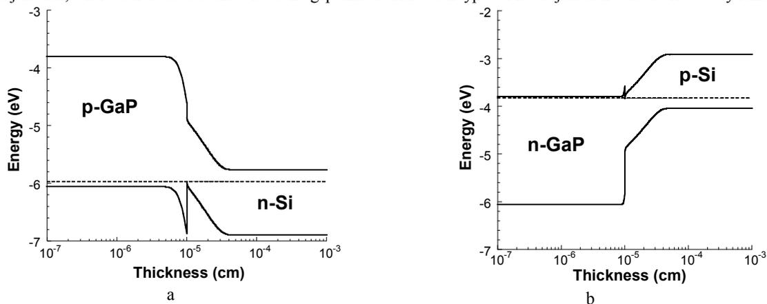
Fig. 1. Calculated band diagram for p-GaP/n-Si (a) and n-GaP/p-Si (b) heterojunctions.
