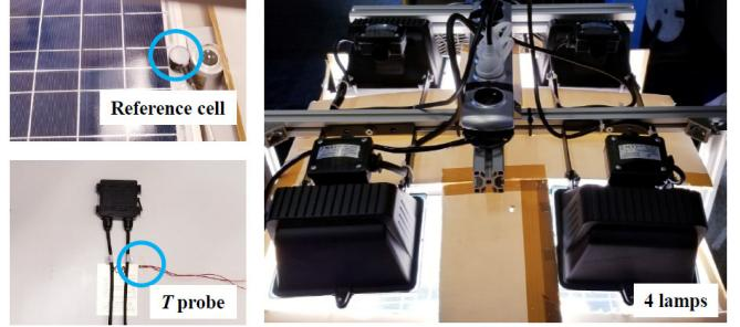
Fig. 1. Experimental setup of indoor controlled -irradiance test
