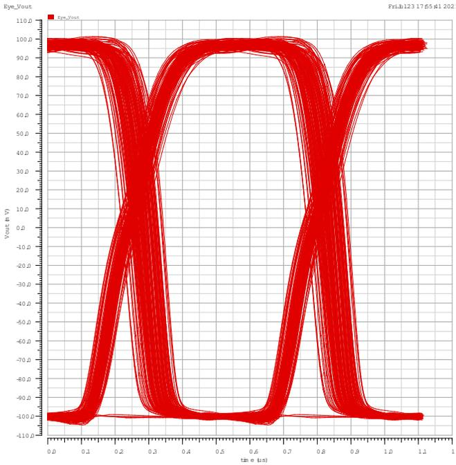
Fig. 5. Eye Diagram of Vout.
