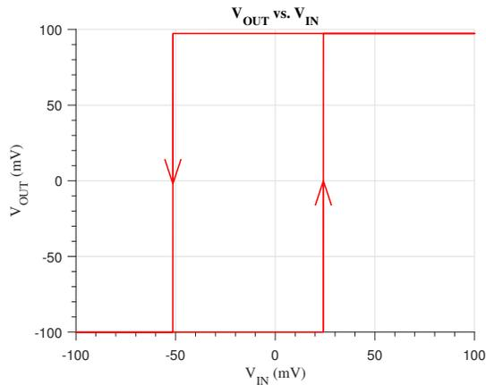
Fig. 4. Post-layout simulation  $V_{IN}$  vs  $V_{OUT}$  hysteresis cycle.
