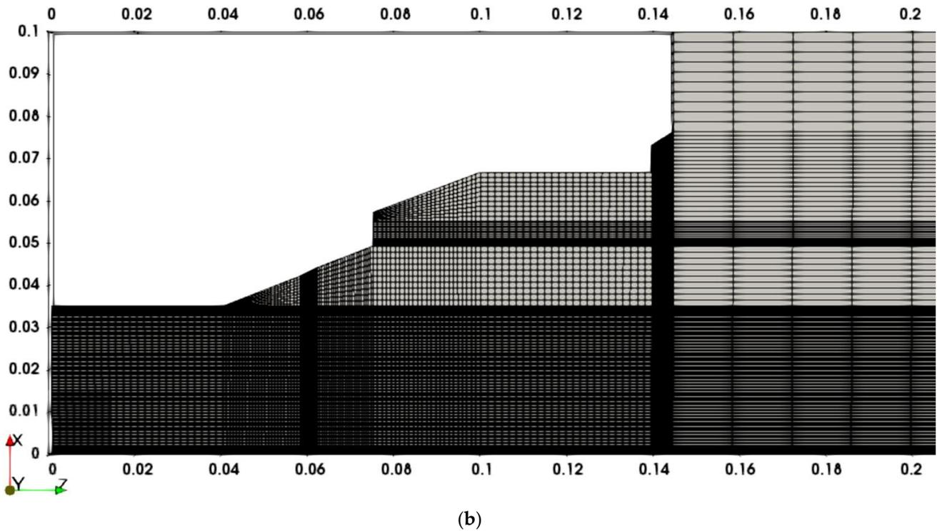
**Figure 1.** (a). General view of the reactor bed design (Salome) and 2D wedge mesh (OpenFOAM). (b). A sketch of the meshed down part of the reactor bed prepared in 2D wedge (length unit is the meter).
